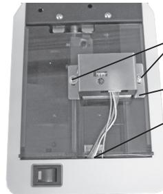
2xM2.6 screws with washer, attach to the acrylic cover.
