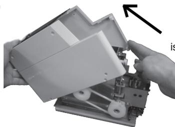
Please remove the body cover slowly at an angle, as the power switch wire is still attached to the main mechanical body.
